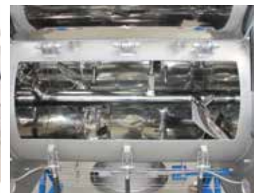
304L / 316L stainless steel internal polishing
